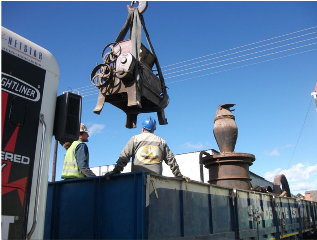
It was driven by a Crossley X producer-gas engine, which was also recovered:
