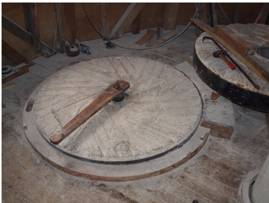
Checking the eastern Stone Spindle for verticality using the Trammel
